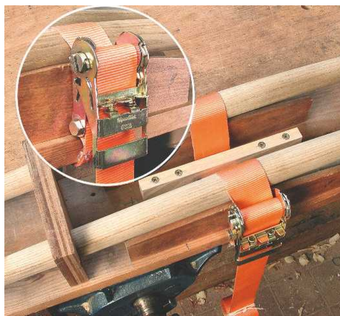
▲ Pic. 3 The central divider helps to fold the webbing round the legs
